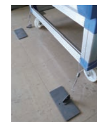
The earthquake damaged the earthquake-resistant fittings of this chemical storage cabinet.
