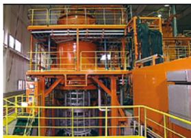
Vertical single-chamber vacuum furnace (Japan's largest)
