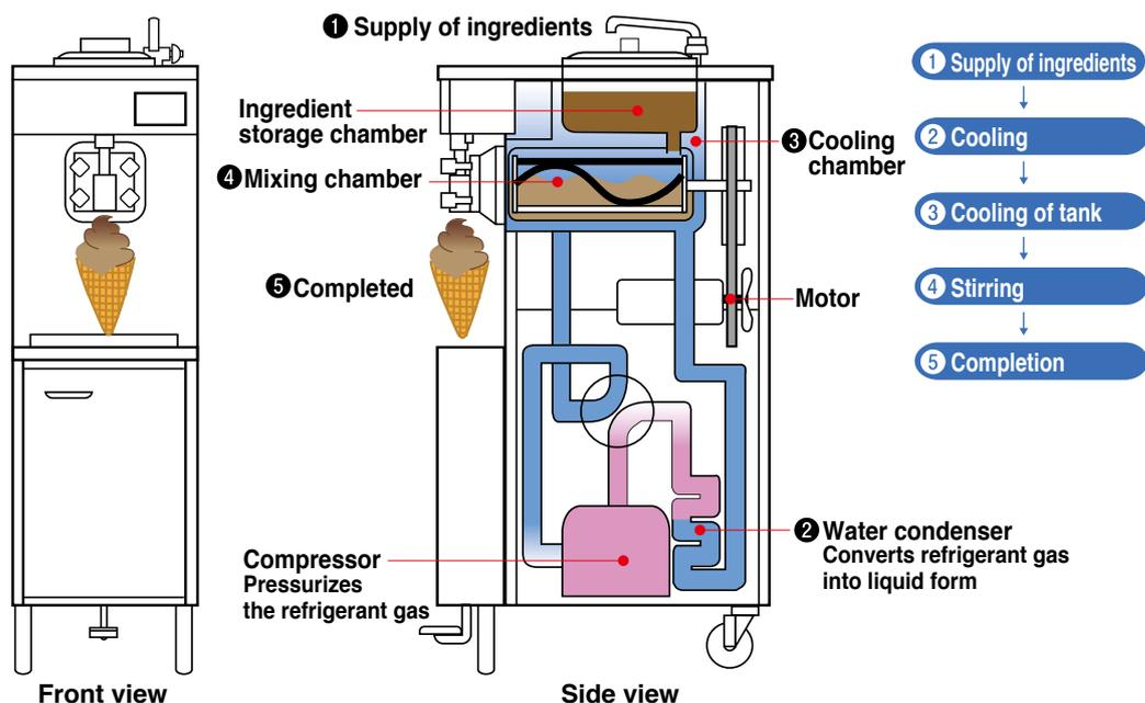
Figure 1: Mechanism of a soft serve freezer
