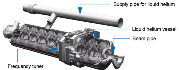
**Figure 6: Superconducting acceleration cavity unit**
