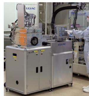
ULVAC, Inc. has developed its S-QAM series of complex sputtering systems for R&D with the aim of delivering maximum performance at a minimal cost. Sputtering is a vacuum deposition method that is used in the manufacture of semiconductors, electronic parts and
