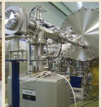
An ideal vacuum is essential in accelerators. This photo shows an ULVAC ion pump.
