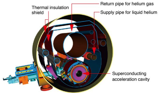
**Figure 7: Cross section of cryomodule**
