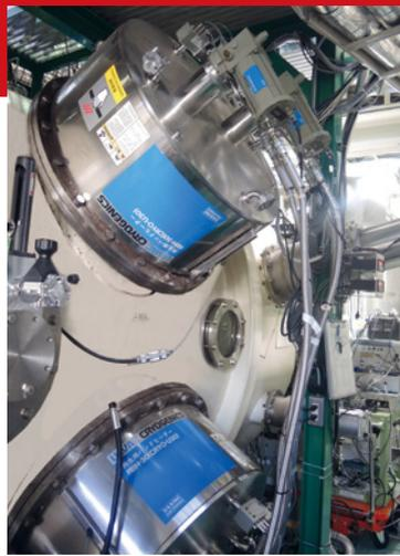
The cryopump incorporated in the space chamber, which played an important role in the durability tests (manufactured by ULVAC CRYOGENICS INCORPORATED)
