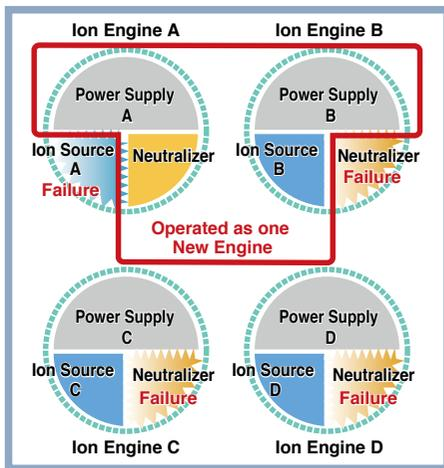
As seen in the figure on the left, the cross operation combines the three undamaged components of ion engines A and B to enable them to operate as a new engine. As a result, the first Hayabusa was able to successfully return to Earth.
