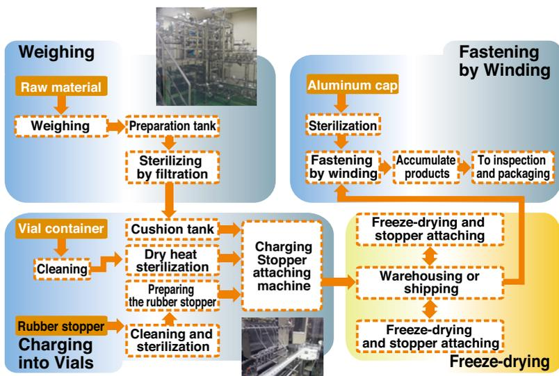
■ Flowchart of process for producing freeze-dried formulation
