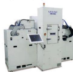
Sputtering equipment for electronic devices
