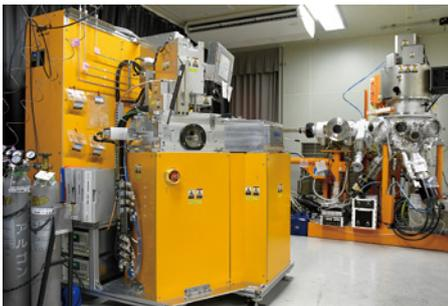
QAM, a compact sputtering system for thin-film deposition R&D
