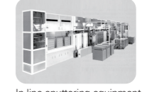
In-line sputtering equipment for magnetic disks
