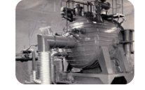
100 kg-class induction heat-type vacuum melting furnace
